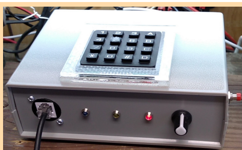
Keypad, embedded in a Lucite® frame, affixed atop Roger KFGBIG 's original ARN-1 case. – Photo by AD6G
